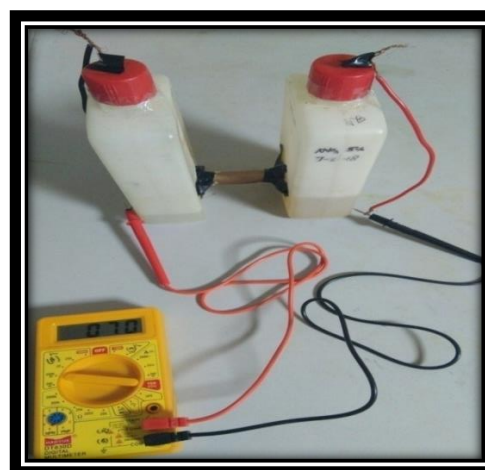
Figure 4: Dual Chambered MFC with Voltmeter
